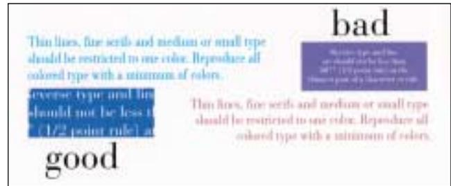
**SWOP 2001's advice on how thick type must be to be knocked out of a screened area leaves much to be desired. Above, the graphic at actual size. Below, a greatly enlarged scan shows how the shapes of the letters were lost in the "good" sample during printing.**
