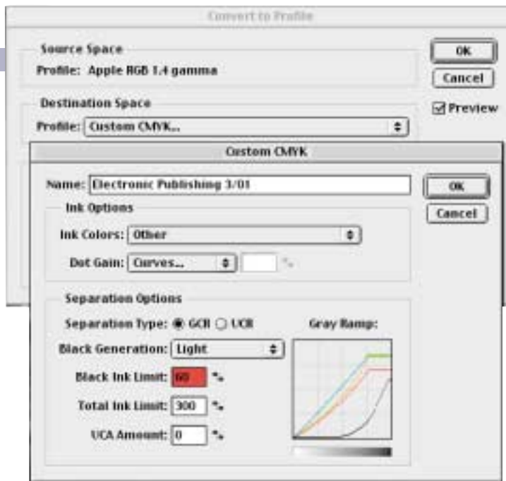
The above dialog creates a custom separation. By limiting the black channel to a maximum of 60%, it creates a black that seems absurdly light, below.
